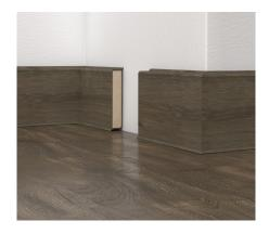
Consisting of HDF - core, covered with the chlorine-free polyblend based on PP/TPE, with flexible edges on top and bottom
