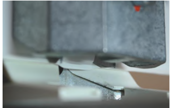
1 turn over the profile on the head - put it straight on the trestle - lock the clamping device - cut very carefully
