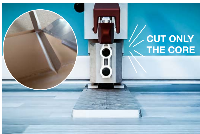
Notch very carefully: Stop when the resistance decrease
