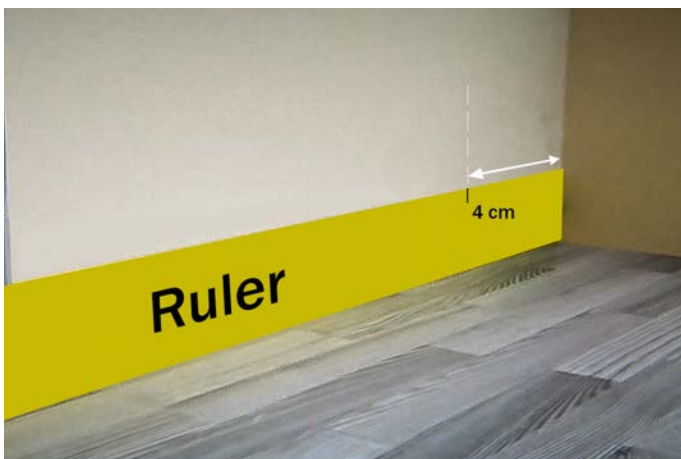
Position a normal ruler behind the skirting at the corner
